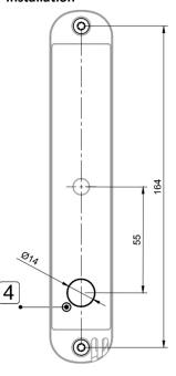
Mount the display in the area of the benches and keep a distance of at least 15 cm between the cabin ceiling and the upper edge of the device. Keep a minimum distance of 1 meter from the heater.
