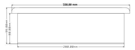
L x W x D = 330 x 310 x 96 mm; light-emitting surface = 250 x 250mm;  $\sim 3000$  g without cable and loose; differences possible depending on customer finish
