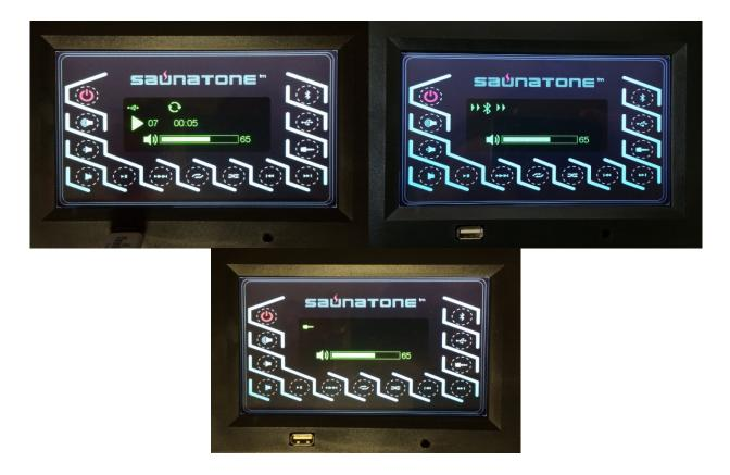
After a few seconds the Audio screen will automatically go back to the Sauna Control screen. You will now see an icon in the middle of your screen displaying the audio function that is still operating in the Audio screen.
