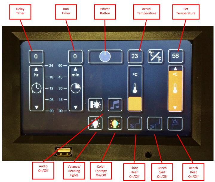
**Main Power:** Press **POWER** button in the upper middle portion of the screen. When lit red, control is **ON**. When white, control is **OFF.**
