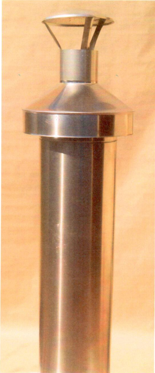
Photo 14. Element for testing rain water durability of the three-wall chimney system type "SKDTŻ-3L".
