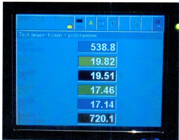
Photo 11. Measurement of outer wall temperature during thermal tests of the three-wall chimney systems type "SKDTŻ-3L".
