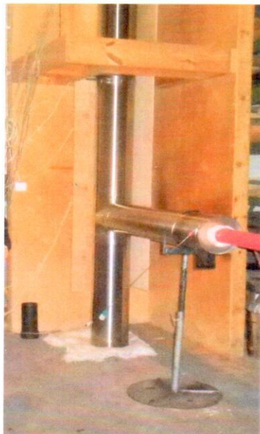
Photo 12. The course of the test of resistance to fire at the workstation according to standard PN-EN 1859.
