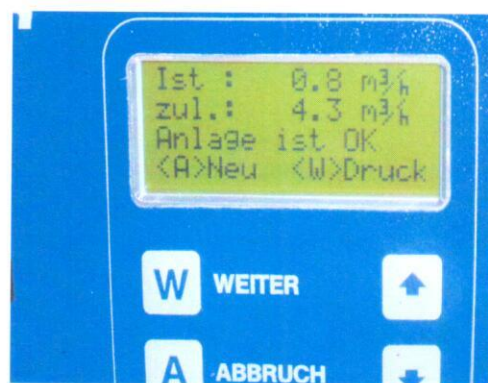
Photo 4. Course of gas tightness test of three-wall chimney systems type “SKDTŻ-3L”.
