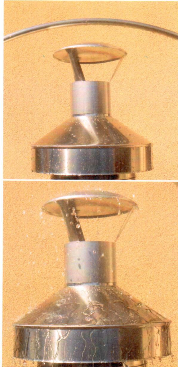
Photo 15. The course of the rain water durability test of the three-wall chimney systems "SKDTŻ-3L".
