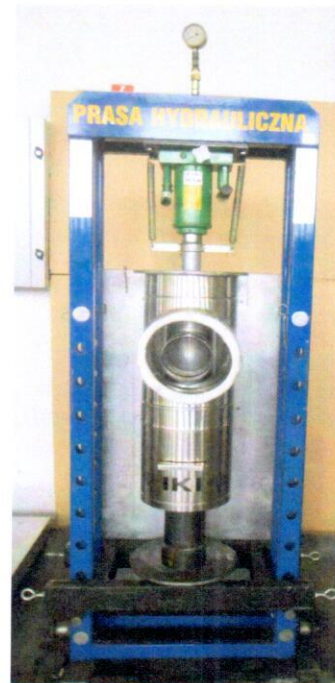
Photo 7. The course of the compressive strength test of the three-wall chimney system type “SKDTŻ-3L”.
