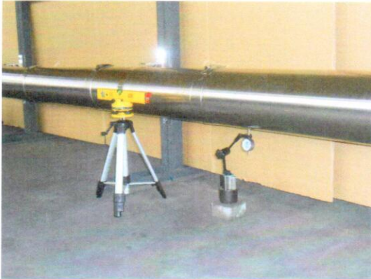
Photo 5. The course of the wind load mechanical properties test.
