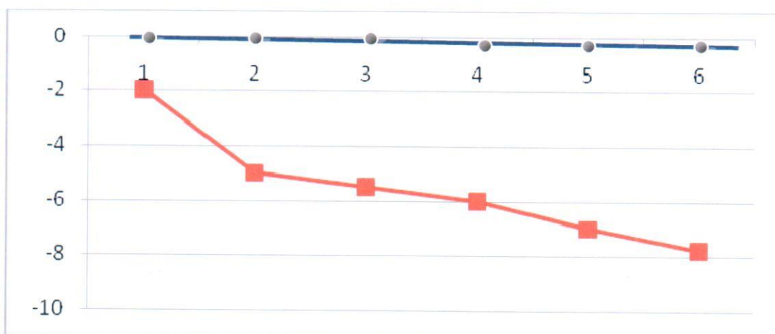
Fig. 3. Diagram of deflections of three-wall chimney systems type “SKDTŻ-3L” upon wind load strength test, where:
